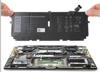
Remove the battery from its recess.
