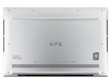
Use a T5 Torx screwdriver to remove the eight 3.3 mm screws securing the case.
