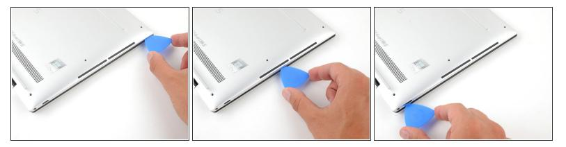
Continue sliding the opening pick along the perimeter of the lower case to release the remaining clips.
