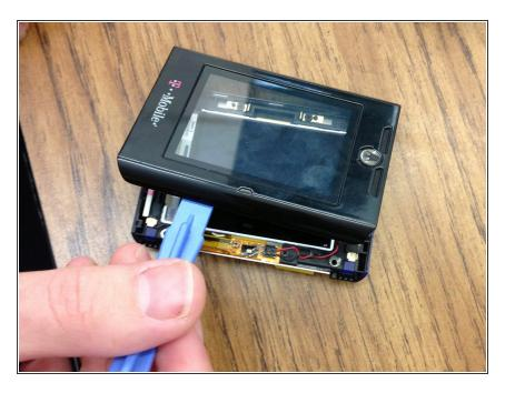
Use the plastic opening tool to pry the protective screen off the main part off the screen.
