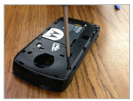
On the back of the device unscrew the top right, top left, bottom right, and bottom left buttons using appropriate size Phillips screwdriver.
