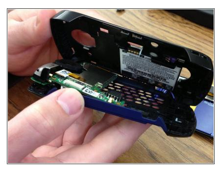
Once screws are dismantled, use plastic opening tool to assist separation of the top half of device from the bottom half.
