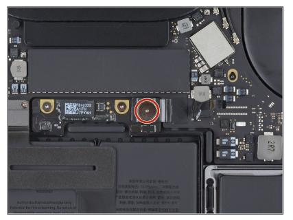
Use a T5 Torx driver to remove the 3.7 mm pancake screw securing the battery power connector.
