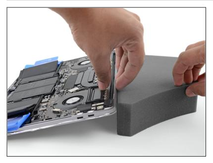
Next, raise the back edge of your MacBook Pro to direct the flow of adhesive remover away from the keyboard/logic board area.
