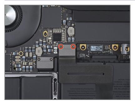
Use a T3 Torx driver to remove the two 1.8 mm screws securing the trackpad cable connector bracket.
