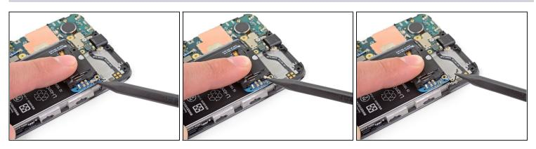
Use the tip of a spudger to disconnect the antenna flex cable from the loudspeaker assembly.
