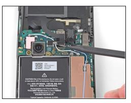
• Use the tip of a spudger to disconnect the two flex cables connecting the fingerprint sensor and buttons to the motherboard.
