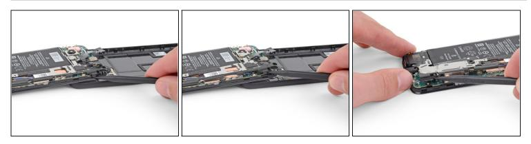
• Use the tip of a spudger to unclip the motherboard bracket from the upper-right and lower-right corners of the motherboard.
