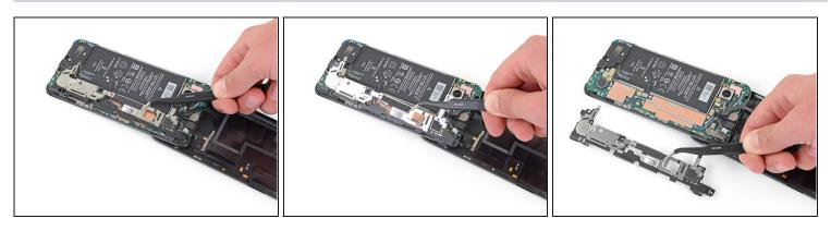
• Use a pair of <u>tweezers</u> to remove the motherboard bracket.
