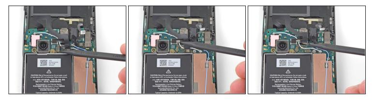
• Use the tip of a spudger to disconnect the two flex cables connecting the fingerprint sensor and buttons to the motherboard.
