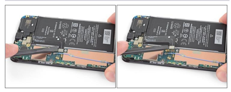
• Use the flat end of a spudger to pry up and disconnect the battery cable.
