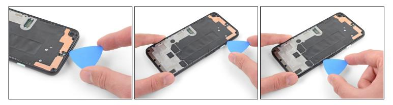
• Slide the opening pick around the top and right edges of the phone to release the rest of the clips.
