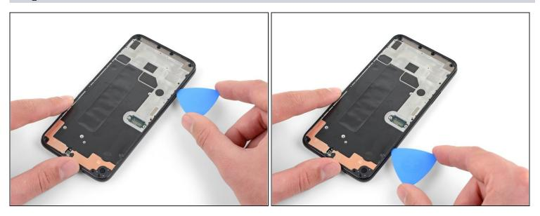
• Slide the opening pick around the left edge of the phone to release the plastic clips securing the back cover to the midframe.
