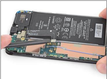
• Use the flat end of a spudger to pry up and disconnect the battery cable.
