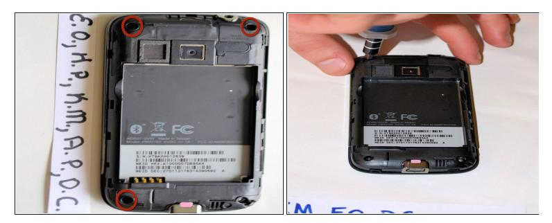
• Use the T4 screwdriver to remove the three .05 mm screws from the back cover.
