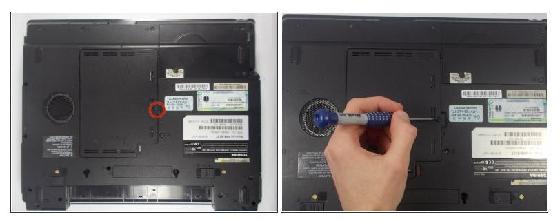
Loosen this 5 mm Phillips #0 screw found in the center of the lower case.
