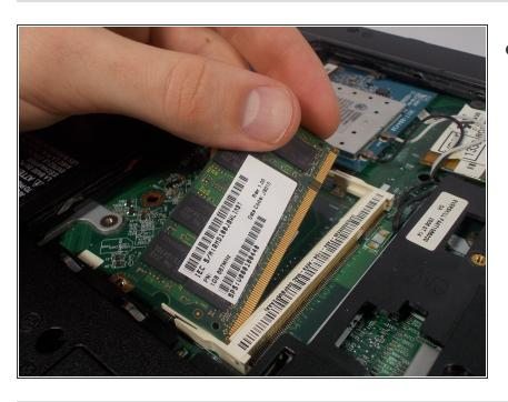
Pull the RAM out of the dock by lifting it from the left side and sliding it towards the left.
