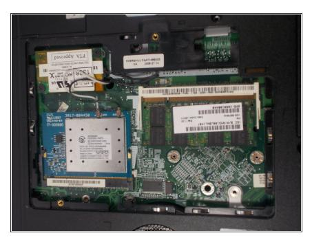
The computer should be open with many of the internal components shown. You can now access the RAM, and wireless card.
