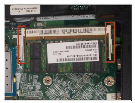
Push the two white tabs away from the RAM. The left side of the RAM should pop out of its holder.
