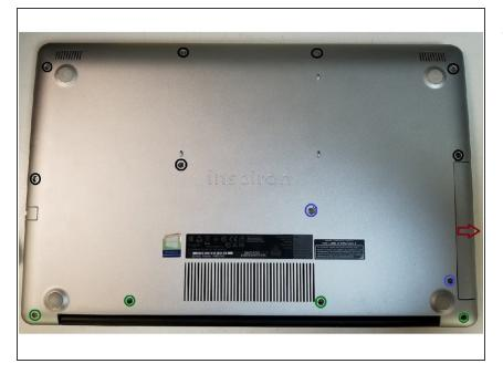
With both screws marked in purple removed, now slide out the disk drive, as marked with the arrow, to reveal the remaining, hidden pair of screws holding the backplate on.
