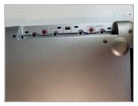
Underneath the optical drive are two final screws preventing removal of the backplate. Remove both of the screws marked in red.
