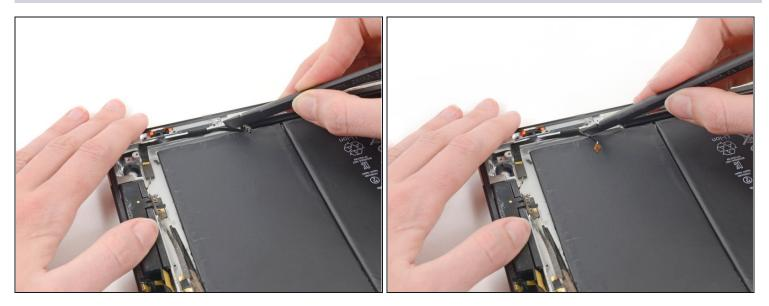
• Slide a spudger underneath the power & volume cables, releasing the adhesive.
