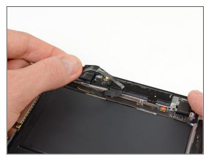
• Peel back and remove the adhesive tape covering the headphone jack assembly.
