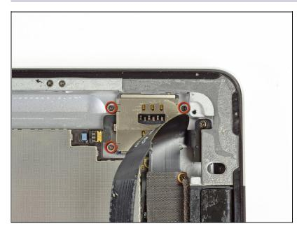
Remove the three 1.75 mm Phillips #00 screws securing the SIM board to the aluminum frame.
