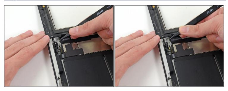
• Use a pair of tweezers to pull the home button ribbon cable straight out of its socket on the logic board.
