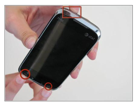
With the phone powered off, press and hold the Talk/Send, End, and Power buttons (the 3 circled here) for about 3 seconds.
