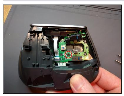
Remove the single Phillips screw holding the top chassis motherboard to the top chassis.
