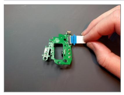
Use a plastic spudger to pivot the lock on the ribbon cable connector, then remove the ribbon cable from the connector.
