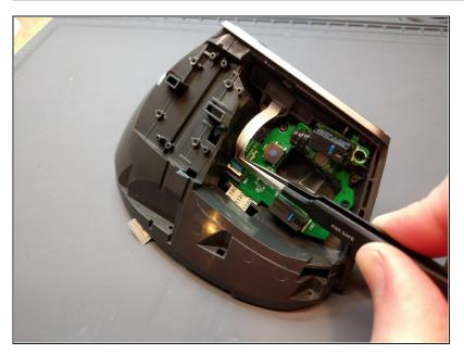
Use a plastic spudger to pivot the lock on the ribbon cable connector for the navigation button assembly, then lift the ribbon cable out of the connector.
