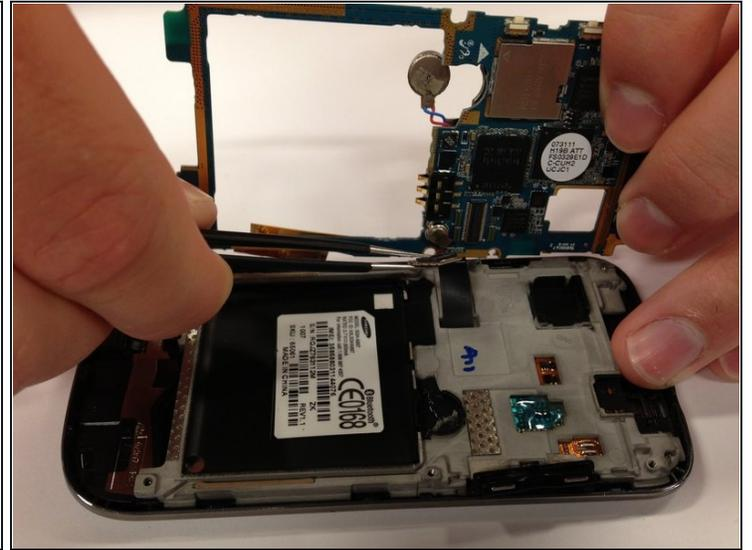
**⚠ DO NOT** remove the motherboard completely. One more clip on the motherboard's backside needs to be removed.
