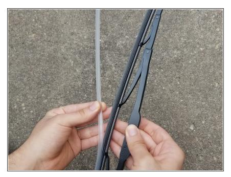
Remove the plastic protection from the rubber side of the new wiper blades.
