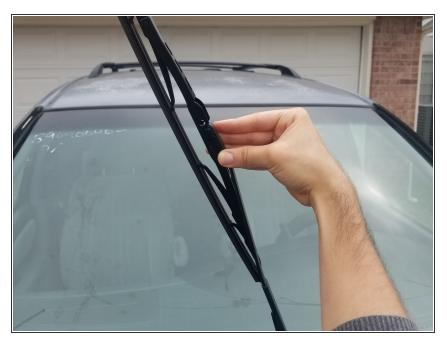
• Lift the windshield wiper to a 90degree angle above the windshield.
