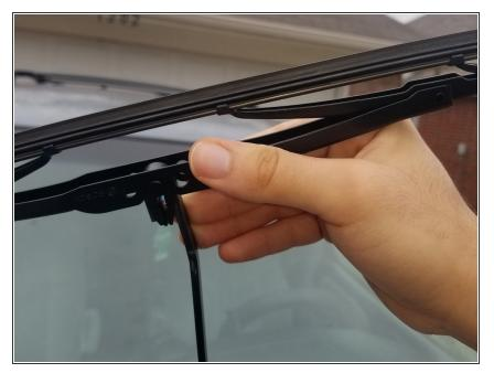
• Lift the wiper arm back up and latch the j-hook around the mounting point of the new blade.
