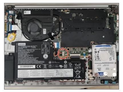
• Using a spudger gently push the plastic connector to the left in order to disconnect the battery.
