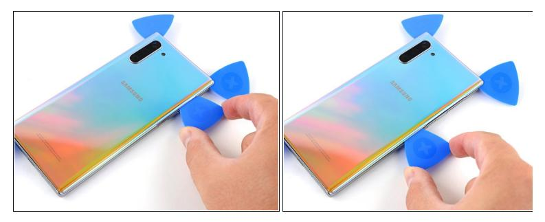
• Insert a fourth and final opening pick into the gap on the right side of the phone, sliding it down towards the bottom right corner of the phone to slice the adhesive.
