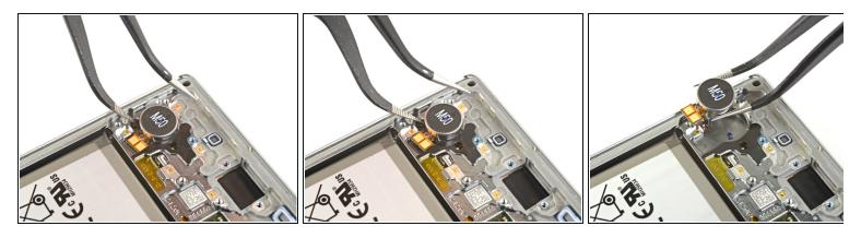
• Use one side of a pair of tweezers to reach underneath the vibration motor using the gap in the frame near the bottom right corner of the battery.
