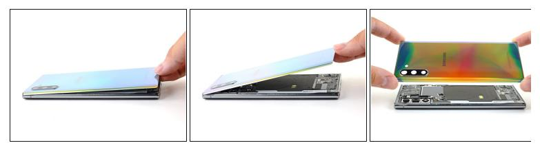
• Lift up and remove the back panel.
