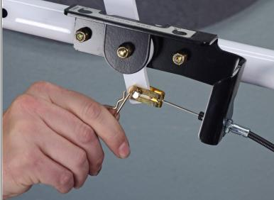
Remove the cotter pin from the clevis.
