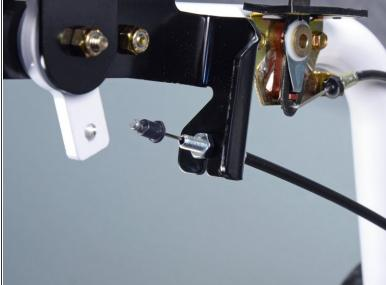
• Use a 7/16 inch wrench to unscrew the nut securing the cable housing to the bracket.
