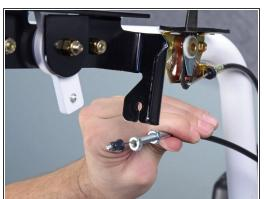
Slide the cable housing out from the deflector lever bracket.
