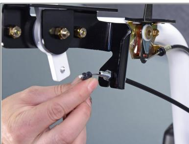
Slide the rubber boot off of the cable housing to the end of the cable.
