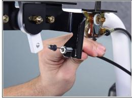
Slide the cable housing back onto the deflector lever bracket.
