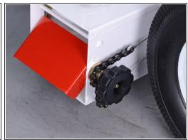
Drop the middle link onto the middle tooth of the pivot.
