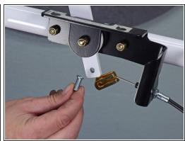
Remove the clevis pin.
