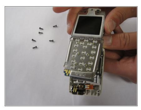
Once the screws have been removed, the front plate of the phone should be removed, exposing the inside electronic components of the phone.
