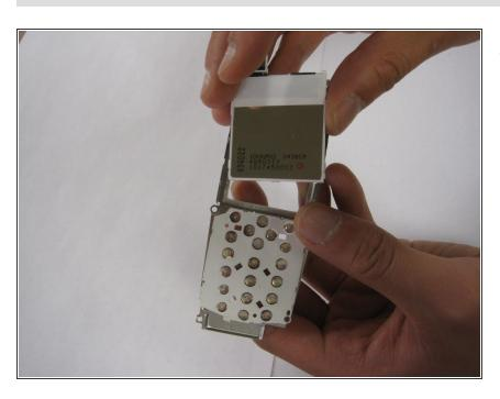
The LCD screen can now be removed from the body of the phone.
