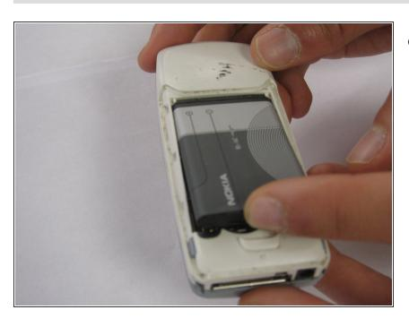
Once the back cover plate is removed, the battery should be exposed. Remove the battery by prying it out. This can be done with your finger-nail or a prying tool.
