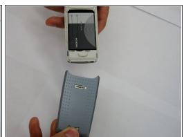
Remove the back cover plate of the phone. To do this press down the lock as you slide the cover toward the bottom of the phone.
