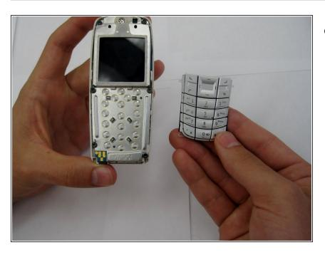
Once the cover plate has been removed, the keypad should easily pop out.
