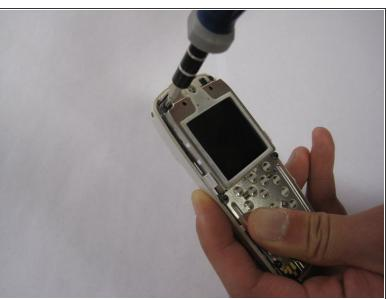
Using a screwdriver, remove the 6, 7 mm Torx-head screws on the front of the phone.
