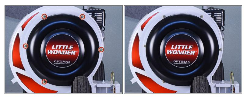
Use a 1/2 inch socket to remove the five bolts securing the intake guard.
