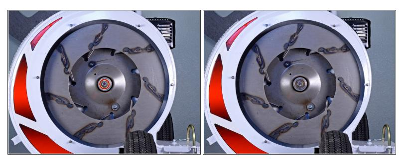
• Use an impact wrench to remove the 5/8 inch bolt securing the fan blade to the spindle.
