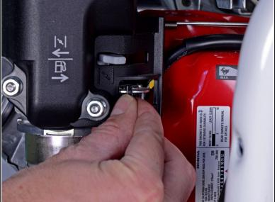
Locate the gas cutoff valve and flip the switch to the left to shut it.
