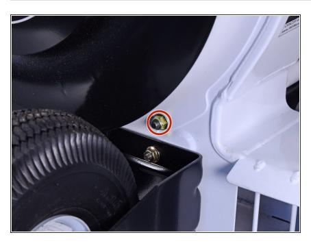
Use a 1/2 inch wrench to remove the intake guard bolt behind the front wheel.
