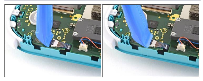
• Use an opening tool or your fingernail to flip up the small, hinged locking flap on the right joystick cable's ZIF connector.
