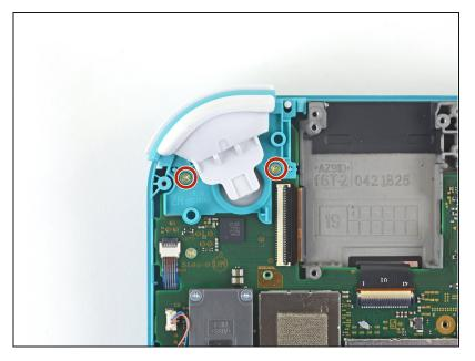
Use a JIS 000 driver or an official iFixit PH 000 driver to remove the two 4.5 mm screws securing the right trigger button assembly to the motherboard.
