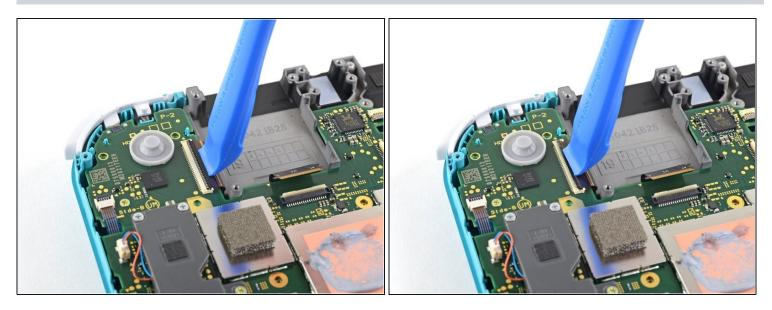
• Use an opening tool or your fingernail to flip up the small, hinged locking flap on the digitizer cable's ZIF connector.
