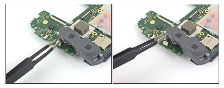
• Use a pair of tweezers or your fingers to pull the right speaker cable straight up and out of its socket on the motherboard.
