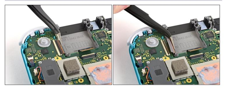
• Use a pair of tweezers to slide the digitizer cable out of its connector on the motherboard.
