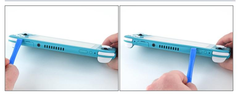
• Continue sliding and prying the opening tool along the gap on the top of the device to release the clips.
