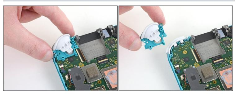
• Remove the right trigger button assembly.
