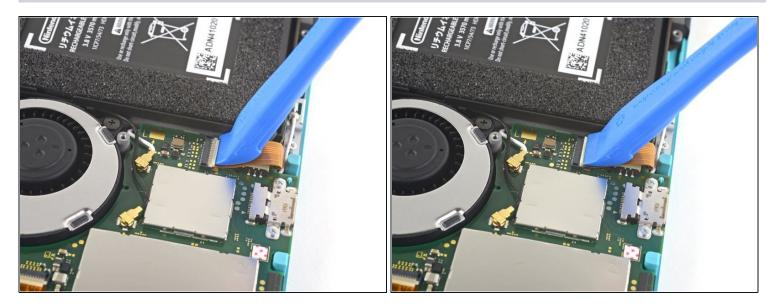
• Use an opening tool or your fingernail to flip up the small, hinged locking flap on the motherboard interconnect cable's <u>ZIF connector</u>.
