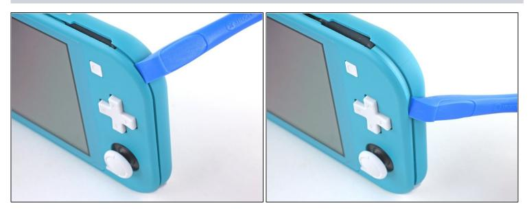
Slide the opening tool around the bottom-left corner to release the clips on the left side of the device.
