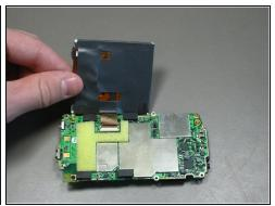
Lift up the LCD screen so that the ribbon strip connecting it to the motherboard can be accessed.
