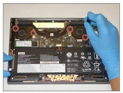
• Remove the four 3 mm Phillips #0 screws from the fan assembly.
