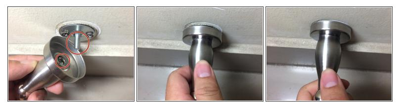
• Attach the anchor fitting into the mount base by rotating it clockwise.
