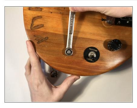
Using an 11 mm wrench, remove the nut of the tone control.
