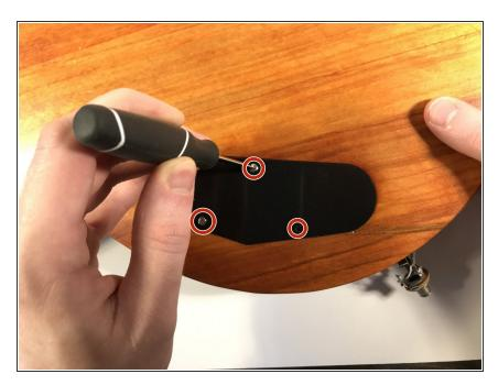
With a Phillips #1 screwdriver, remove the three 7 mm screws holding on the back plate.
