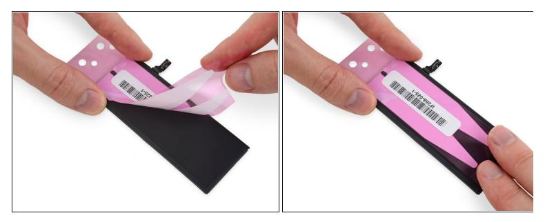
Lay the strips down flat on the back of the battery.
