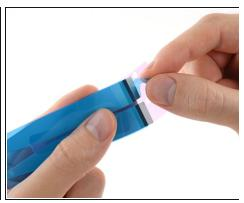
Remove the small sections of blue film covering the flat ends of the adhesive strips. Don't remove the entire blue liner, just the small parts covering the pull tabs.
