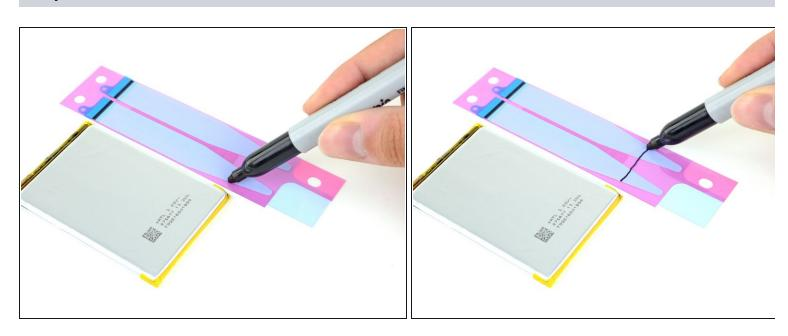
Using a pen, mark a line on the stretch release adhesive just slightly above the bottom edge of the battery.
