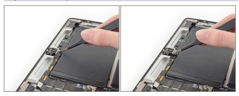
• If present, remove the piece of tape covering the end of the front facing camera cable with a pair of tweezers.
