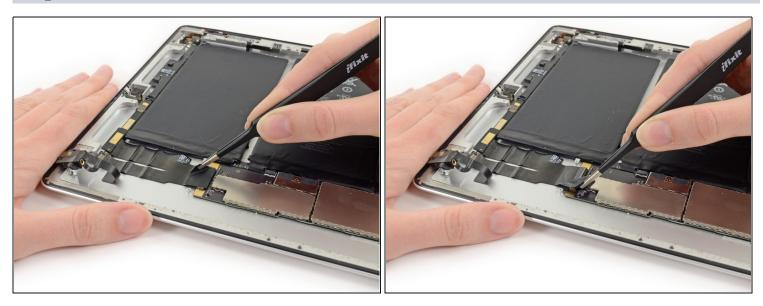
• If present, use tweezers to remove the piece of tape covering the end of the headphone jack/control board cable.
