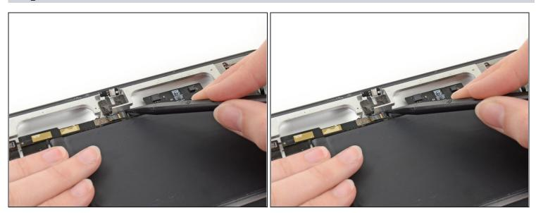
• Use the flat end of a spudger to flip up the retaining flap on the microphone ribbon cable ZIF socket.
