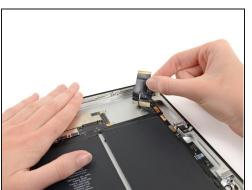
• Gently peel the headphone jack/control board ribbon cable away from the rear case to free it from the adhesive.
