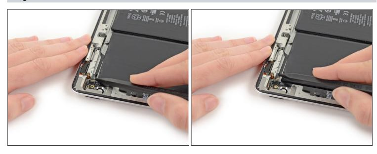
Run the tip of a spudger underneath the button assembly cable to free it from the socket.
