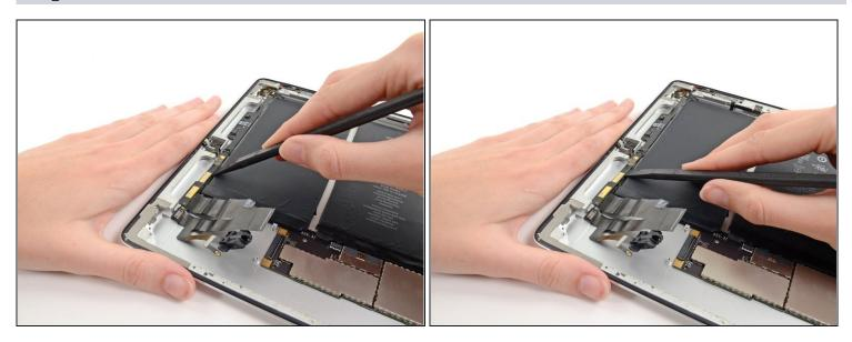
• To begin freeing it from adhesive, pry gently under the control board near the front-facing camera socket.
