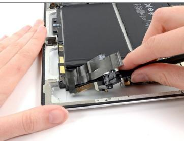
• Slide the flat end of a spudger under the middle portion of the ribbon cable to separate the adhesive holding it to the rear case.
