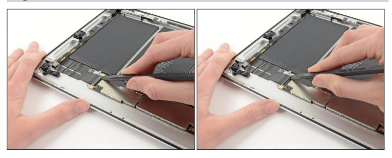
• Use the flat end of a spudger to flip up the retaining flap on the headphone jack/control board cable ZIF socket.
