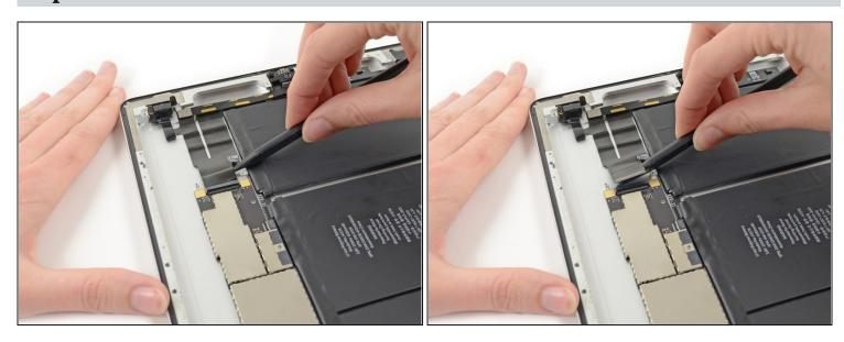
• Slide the tip of a spudger underneath the headphone jack/control board ribbon cable to disconnect it.
