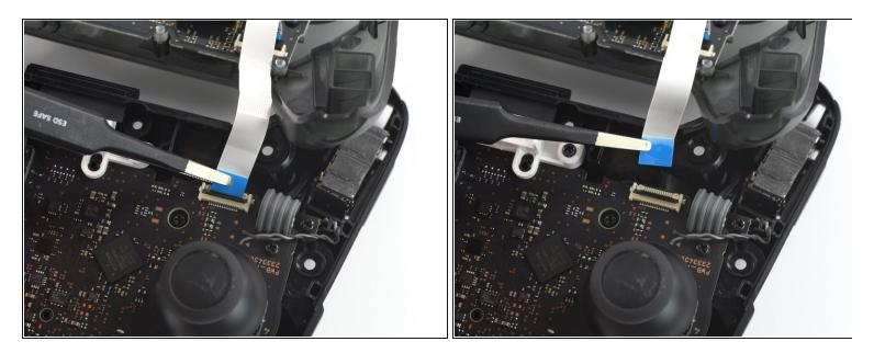
• Use your fingers or a pair of blunt nose tweezers to disconnect the interconnect cable from its connector.
