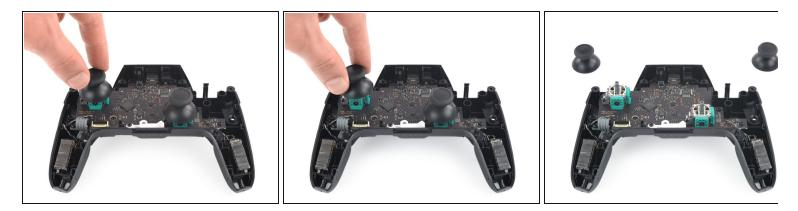
• With light force pull the two joystick caps off of the controller.
