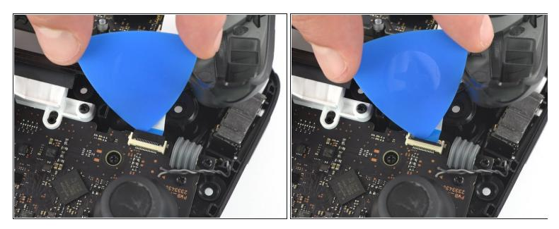
Use the tip of an opening pick to open the black flap of the ZIF connector by pushing it upwards.
