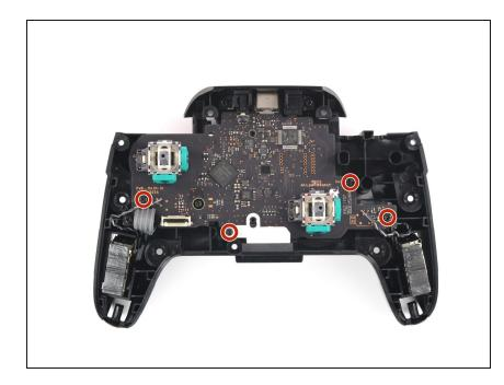
Use a Phillips screwdriver to remove the four 5 mm-long screws securing the motherboard.
