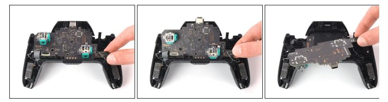
• Lift the motherboard carefully as to not damage the wires and flip it to reveal the backside.
