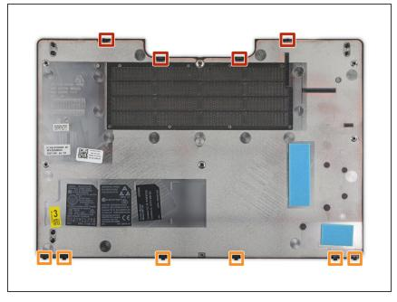
i This photo shows the location of the ten clips that hold the lower case in place. Take note of the location of
