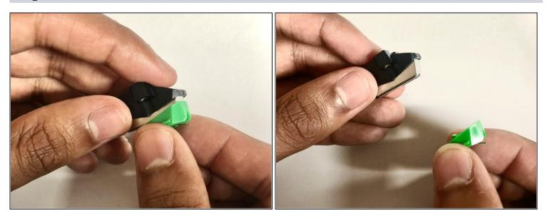
• Pull the needle off of the new cartridge to ensure it does not get damaged during installation.
