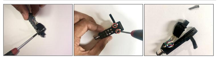
• Use a <u>2.5 mm flathead</u> screwdriver to remove both screws from the headshell.
