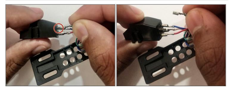
• Gently pull the four wires out from the back of the cartridge.
