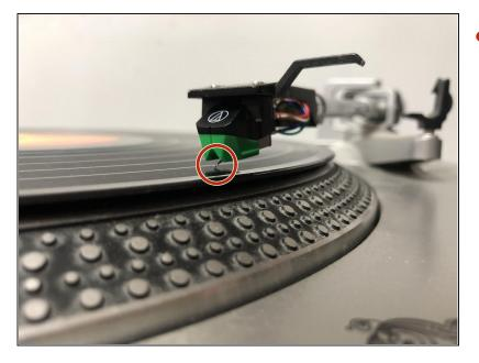
Place the needle onto a vinyl record and ensure that only the tip of the needle is touching the record and not the cartridge.
