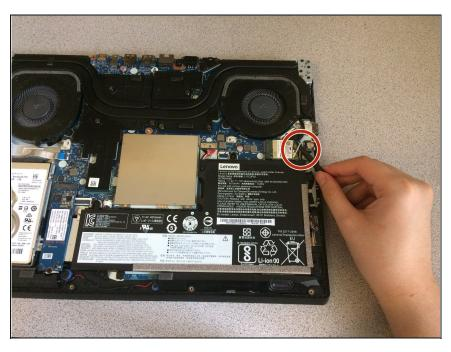
Detach the two antenna wires attached to the wireless LAN card.
