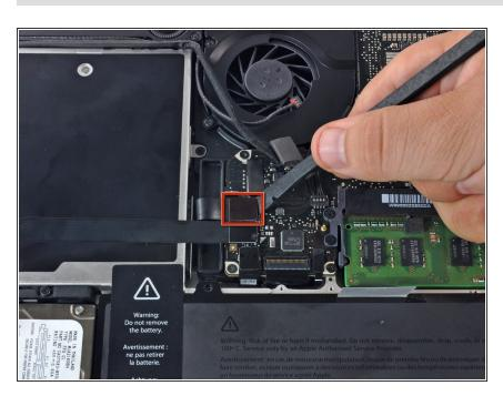
Use the flat end of a spudger to pry the optical drive connector straight up off the logic board.
