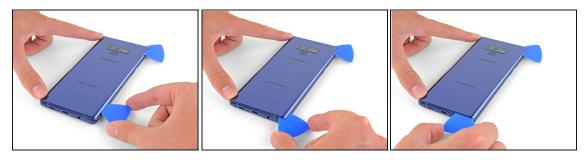
A Be careful near the corner, as the glass is very weak. Apply more heat at any time if the adhesive becomes stuck.
