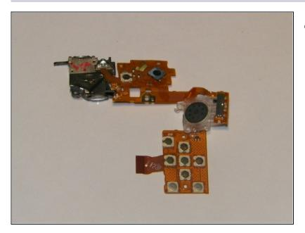
The rear control board should now be completely separate from the camera.
