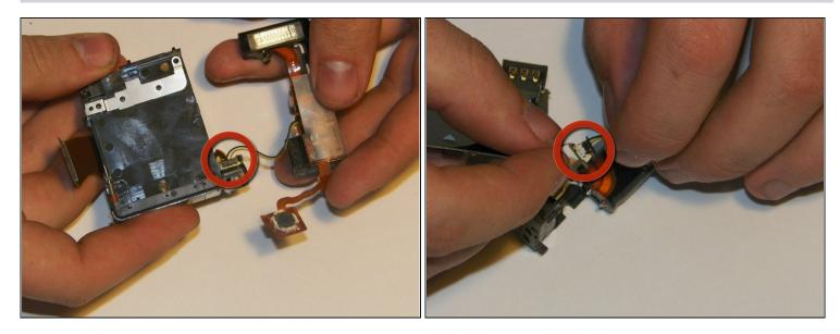
• There is a small connector that mounts in the battery compartment that will need to be unplugged for the flash assembly to be fully removed.
