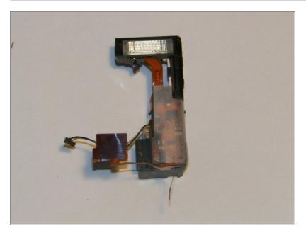
The Flash assembly should now be separate from the rest of the camera.
