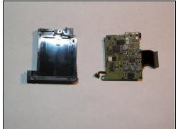
Once the flash assembly has been unplugged and removed, the rear accessory board can simply be pulled up and off of the battery compartment.
