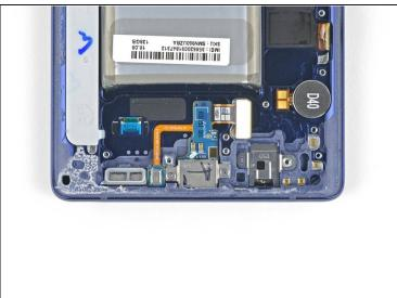
Remove the two 3.2 mm Phillips screws from the charging assembly.
