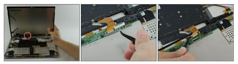
• Begin by removing the ribbon on the right. With the curved tweezers, carefully remove the metal bracket to expose the end of the ribbon. Remove ribbon.
