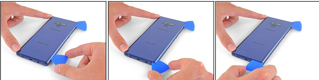
⚠ Be careful near the corner, as the glass is very weak. Apply more heat at any time if the adhesive becomes stuck.
