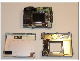
Then, carefully pry apart the front and back outer casing away from the internal components.
