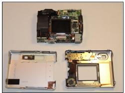
Then, carefully pry apart the front and back outer casing away from the internal components.
