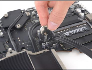
• Pull the PRAM battery straight up and out of its socket.
