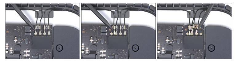
• Use the point of a spudger to pry all four antenna connectors straight up from their sockets and disconnect them from the AirPort/Bluetooth card.
