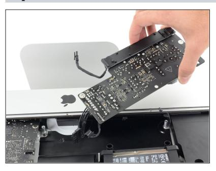
Remove the power supply from the iMac.
