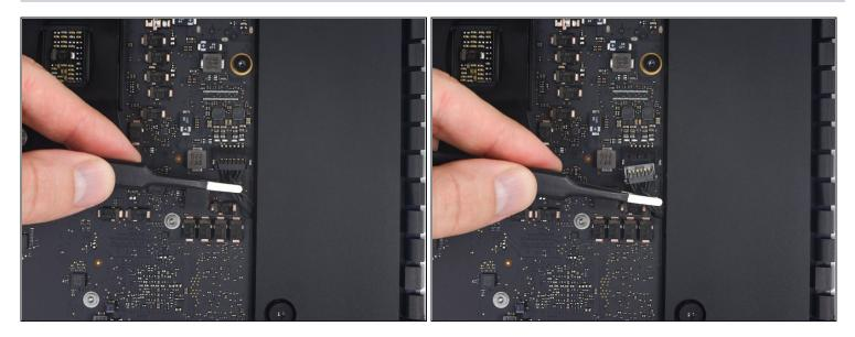
• Use a pair of <u>tweezers</u> or your fingers to pull the right speaker cable connector straight down and out of its socket on the logic board.
