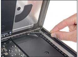
*i* If necessary, a <u>plastic card</u> can be used to cut any remaining sections of the bottom adhesive strip.
