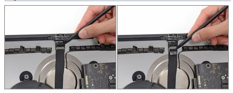
• Use the tip of a spudger to flip down the metal retaining bracket on the camera cable.
