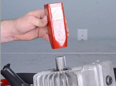
Remove the main shaft adapter.
