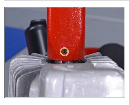
Use a 1/8 inch hex key to loosen the set screw securing the main shaft adapter.
