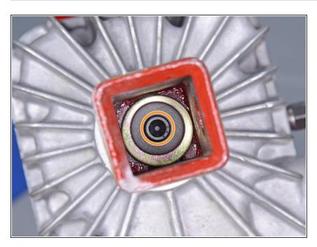
Use a 1/4 inch hex key to remove the bolt securing the main shaft adapter to the main shaft.
