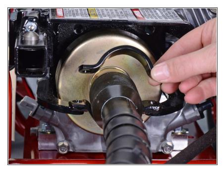
Remove the clutch bracket clamp.
