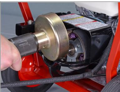
Slide the clutch drum straight off of the clutch rotor assembly.
