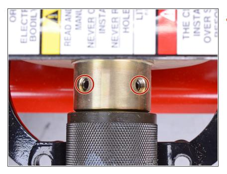
Use a 5/32 inch hex wrench to loosen the two set screws on the clutch drum.
