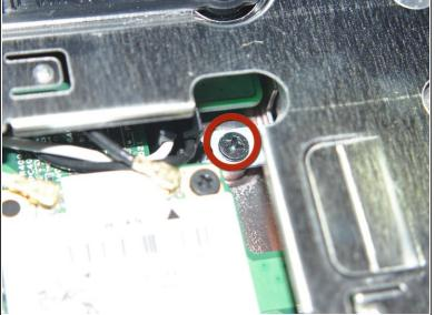
Unscrew the screw next to the wireless card.
