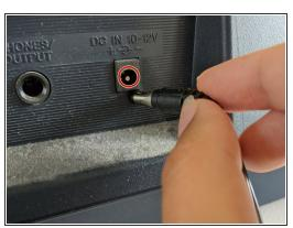
Unplug the cord from the wall and the back of the keyboard.
