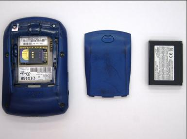
Remove the lithium-ion battery from the back of the device using your index finger.
