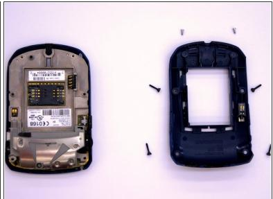
Use the plastic opening tool to pry the back case away from the front case.
