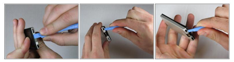
Insert the Zune opening tool between the faceplate and the back cover, starting from the top and slowly work your way around the device.
