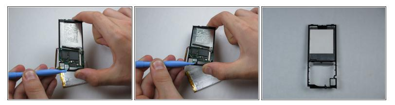
• Pry up the memory board from center piece with a Zune opening tool and gently pull it off.
