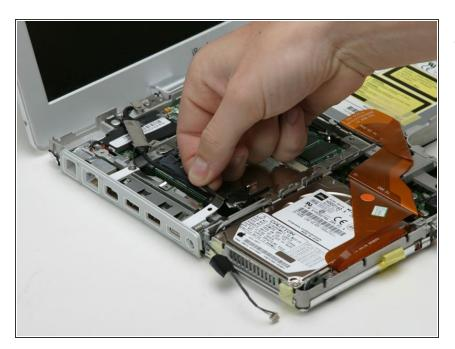
Deroute the display data and microphone cables.
